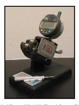
Typical External Variable Thread Gage - "Tri-roll" gage
