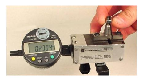
Typical Internal Variable Thread Gage - "Bi-Point" gage
